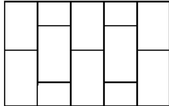
The sheets should also be cut and laid so that the seams do not line up between adjacent rows. Sheets should be butted tightly to each other and the joints can be secured with short strips of duct tape.
