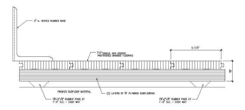
The Zenterra Bamboo Sport Gym Floor is a truly green solution to gymnasium and multi-purpose sports surfacing. It starts with 100% recycled rubber cushioning pads, made of recycled tires. These are fastened to two layers of Forest Stewardship Council (FSC) certified CDX plywood, milled from trees taken from renewable forests. On top of this subflooring is installed bamboo flooring, made from faster growing bamboo plants that may be reused for flooring applications every 5-8 years.
