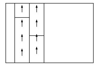
F. Roll material is stretched slightly when it is rolled at the factory. At the job site the installer should allow all rolls to relax for a minimum of two hours before gluing or cutting material.
