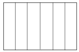
The sheets should also be cut and laid so that any seams do not line up between adjacent rows. Sheets should be butted tightly to each other and the joints can be secured with short strips of duct tape.
