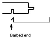
Silver Springs should be spaced about 12"-14" apart, so you will be using six fasteners on the 7' board.
